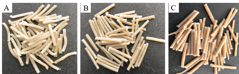
Fig. 2. The appearance of the granules: A – PCL/(AITC/bentonite), B – PCL/(BITC/bentonite), C - PCL/(PEITC/bentonite)).
