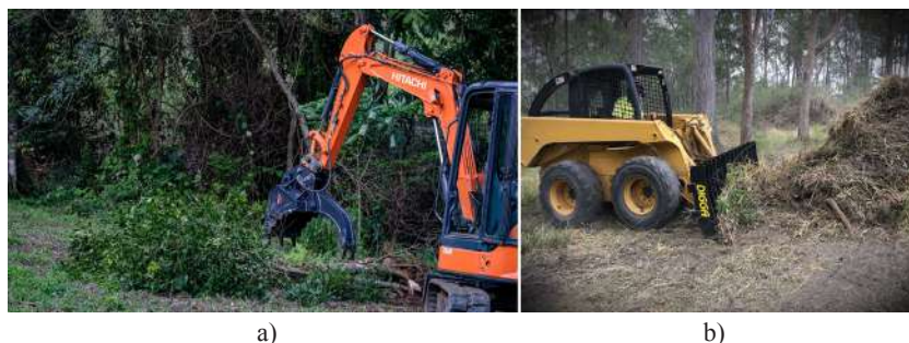
Fig. 2. Collection and raking of logging residues with a forest rake
